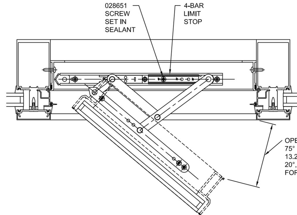
OPENING TO BE APPROXIMATELY 75° MAXIMUM FOR DLO'S OF 13.250 TO 20.499 AND 20°, 30° OR 45° MAXIMUM FOR DLO'S OF 20.500 TO 36.000.
