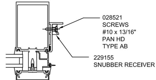
APPLY SNUBBER RECEIVER. USING HOLES IN ADAPTERS DRILL HORIZONTAL WITH #26 DRILL 0.147 DIA. AND APPLY WITH 028251 SCREWS. ADJUST SNUBBER RECEIVER ALL THE WAY TO THE INTERIOR AND SNUG TIGHTEN SCREWS. ADJUSTMENT WILL BE REQUIRED AFTER THE VENT IS INSTALLED.
