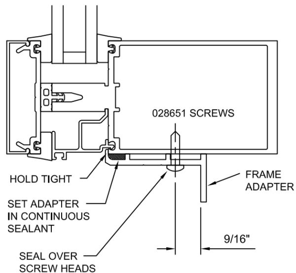
APPLY ADAPTERS TO ALL 4 SIDES AND SEAL CORNERS AS SHOWN.
