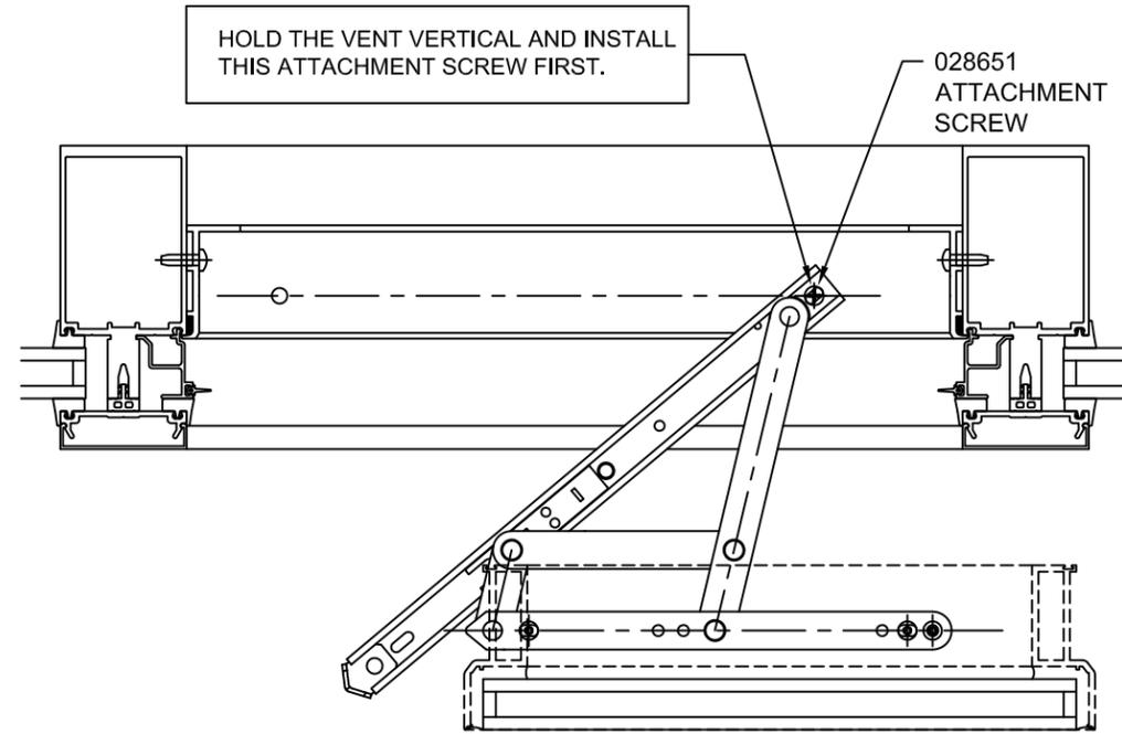
THEN ROTATE THE VENT AND INSTALL THIS ATTACHMENT SCREW.
