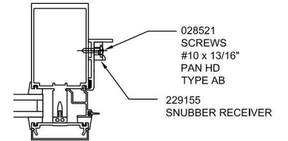
WITH THE VENT OPEN, LOOSEN SCREWS SO SNUBBER RECEIVER WILL SLIDE. THEN SLIDE SNUBBER RECEIVER TOWARDS THE INTERIOR. CLOSE VENT AND LOCK. OPEN THE VENT CAREFULLY AND TIGHTEN SNUBBER RECEIVER SCREWS.
