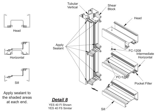
**CAUTION:** Always assemble frames such that each lite of glass will have a minimum of one deep vertical glazing pocket.
