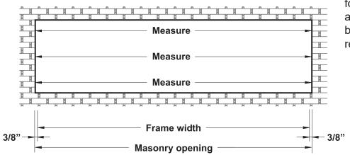
**Note:** Check the opening for squareness and plumb at both ends. Units must be installed in a true rectangle.
