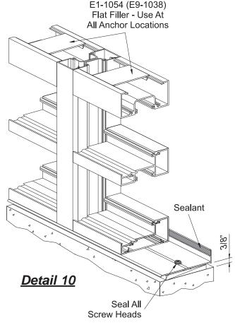
\*Sill anchors penetrate the sill flashing and must be sealed watertight.
