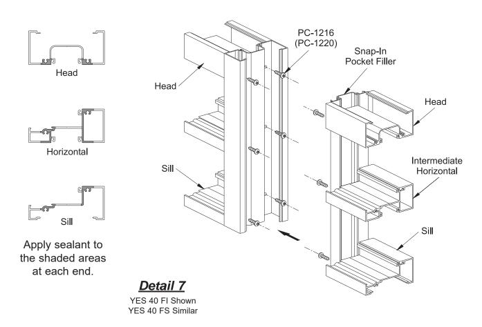
**CAUTION:** Always assemble frames such that each lite of glass will have a minimum of one deep vertical glazing pocket.
