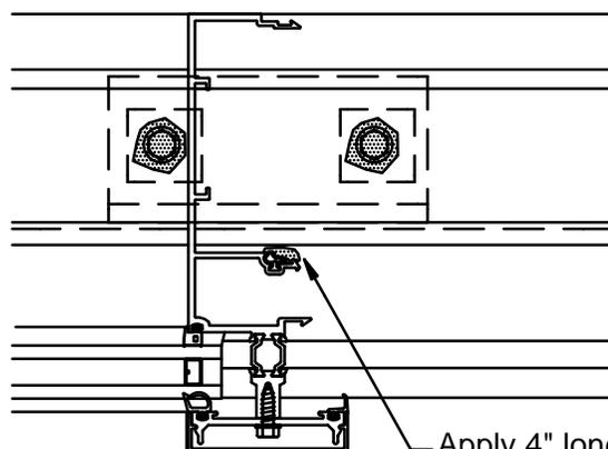
Apply 4" long sealant at the bottom of the mullion along vertical air seal gasket
