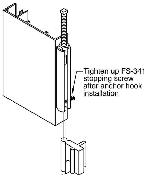
Slide the anchor hook into anchor bracket
