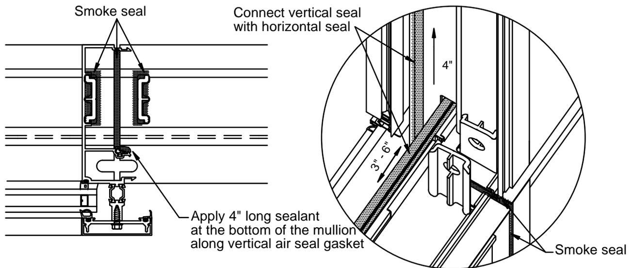
Install the next frame by lifting the frame 4" to 6" above previous frame to clear the sleeves and head horizontals. Move the next frame to the left to engage the outer mullion hooks; then rotate the next frame towards building to snap inner hooks; once snapped, slide the next frame down to engage horizontal air seal at stack joint.
