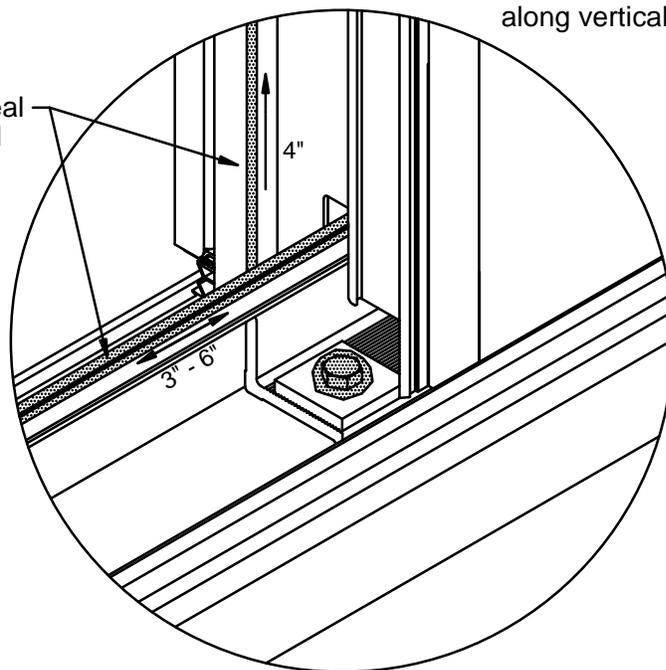
Install the next frame by lifting the frame up to clear the starter sill. Move the next frame to the left to engage the outer mullion hooks; then rotate the next frame towards building to snap inner hooks; once snapped, slide the next frame down to engage horizontal air seal at stack joint.
