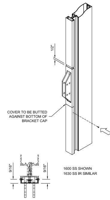
WHEN VERSOLEIL OUTRIGGER SUNSHADES ARE INSTALLED ON THE FOLLOWING CORNER APPLICATIONS, COVER INSTALLATION IS THE SAME AS FOR INTERMEDIATE MULLION LOCATIONS:
