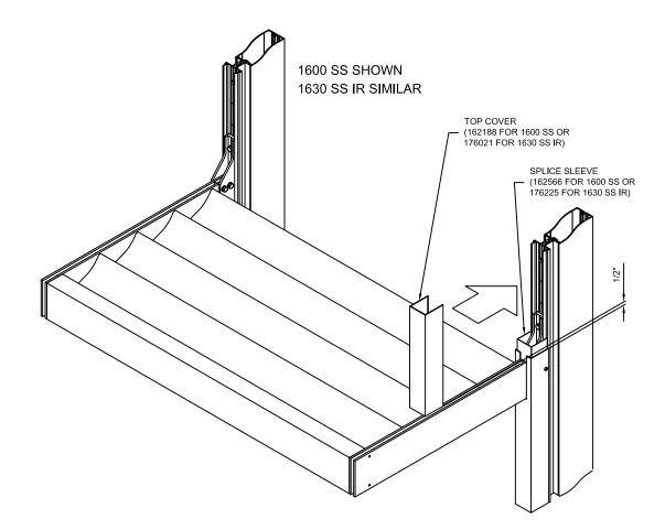
AT ALL VERTICAL COVER LOCATIONS, PIN BOTH HALVES OF THE VERTICAL COVERS. DRILL A Ø0.106" HOLE (#36 DRILL) 2" BELOW THE SPLICE AND 2 7/16" FROM THE OUTSIDE SURFACE OF THE COVER. INSTALL #6 x 3/8" PAN HEAD SCREWS (128920).
