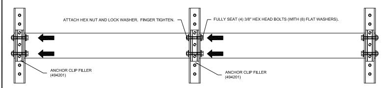
MAKE MINOR ADJUSTMENTS HORIZONTALLY TO ALIGN ALL THE SUNSHADES WHILE TIGHTENING BOLTS AT THE ANCHOR CLIPS. (DO NOT OVER TIGHTEN BOLTS. TIGHTEN TO A SNUG POSITION ENSURING THE SPRING TYPE LOCK WASHERS ARE COMPRESSED. THEN TIGHTEN APPROXIMATELY 1/2 TURN MORE).
