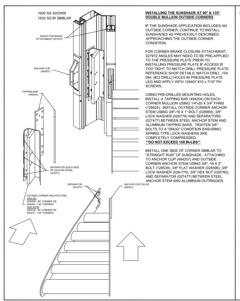
INSTALL SECOND SIDE OF CORNER IN THE SAME MANNER AS THE FIRST, ATTACHING TO ANCHOR CLIP (494207) AND OUTSIDE CORNER ANCHOR STEM USING 3/8"-16 X 2" BOLT (128539), 3/8" FLAT WASHER (028596), 3/8" LOCK WASHER (028779), 3/8" HEX NUT (028780), AND SEPARATOR (027477) BETWEEN STEEL ANCHOR STEM AND ALUMINUM OUTRIGGER.
