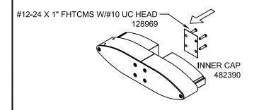
NOTE THAT END ASSEMBLY CAN BE USED AT LEFT JAMB OR RIGHT JAMB (BY ROTATING ASSEMBLY OVER)
