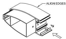
SNAP CONNECTOR END ASSEMBLY (WITH HOLES) AND NOSE END ASSEMBLY TOGETHER
