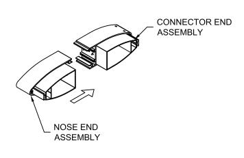
ATTACH ENDCAP TO END ASSEMBLY USING SIX (6) #12-24 X 1" FHTCMS "F" W/#10 UC HEAD (128969) FASTENERS
