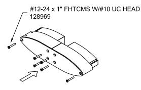
ATTACH INNER CAP (482390) TO END ASSEMBLY USING FOUR (4) #12-24 X 1" FHTCMS "F" W/#10 UC HEAD (128969) **FASTENERS**
