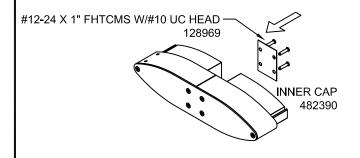
NOTE THAT END ASSEMBLY CAN BE USED AT LEFT JAMB OR RIGHT JAMB (BY ROTATING ASSEMBLY OVER)
