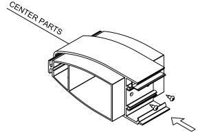
SNAP CONNECTOR SPLICE ASSEMBLY (WITH HOLES) AND NOSE SPLICE ASSEMBLY TOGETHER
