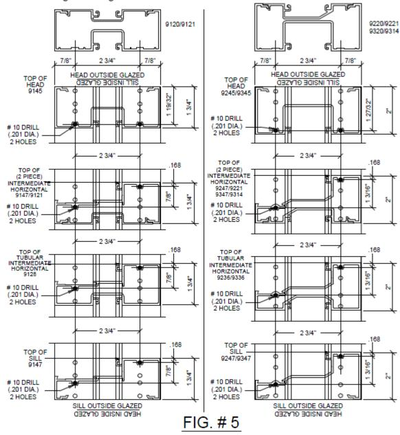
USE BLOCKED OUT HOLE LOCATIONS FOR SCREW SPLINE APPLICATIONS
