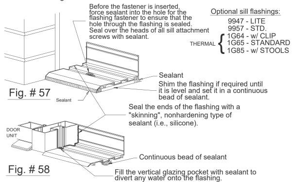
Make sure the bead of sealant under the threshold is continuous through the door jamb and married into the bead of sealant that the sill flashing is set into.
