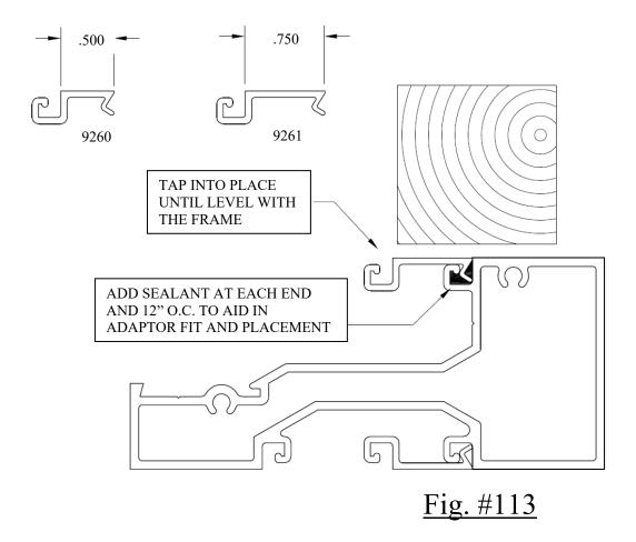
Due to extrusion tolerances and varying thickness of painted finishes, it may be necessary to tap the pocket reducers into place using a hammer and a 6" long block of wood.
