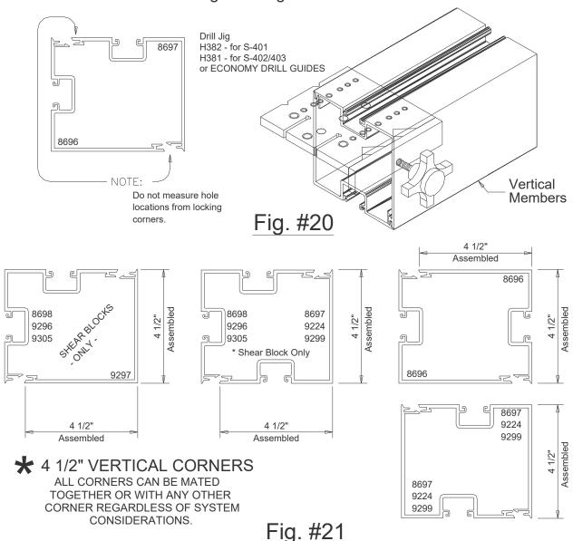
The 90° corner halves may be snapped together and used as a one piece vertical mullion.
