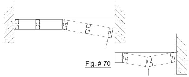
NOTE: If an entrance is required, install the framing units starting at the entrance frame and work towards the end of the opening.
