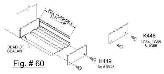
End caps would be incorporated if the sill flashing could not be sealed to the condition completely. An example would be, if the jamb condition was less than the sill flashing depth or a void in the condition exist. This cut length provides a 3/16" gap between the sill flashing and condition for a good sealant joint when end caps are not required.
