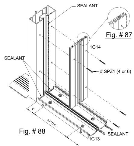
STEP 7) Seal behind the interior half of the verticals (1G14) at the top as shown and attach with (4) or (6) # SPZ3 # 8 X 3/4" PH-SMS as required. See figures above.
