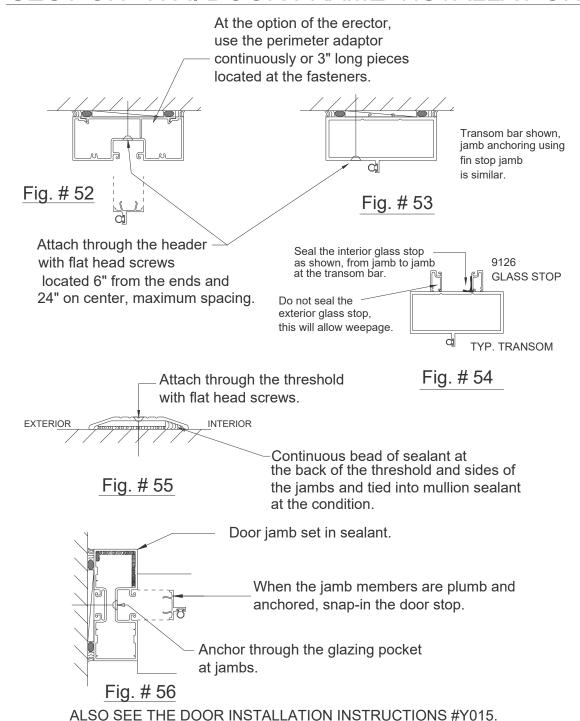
These recommendations are for general erection procedures only. For actual job conditions, see the details on the shop drawings. For perimeter anchor type and spacing, refer to the approved shop drawings or consult the project design professional.
