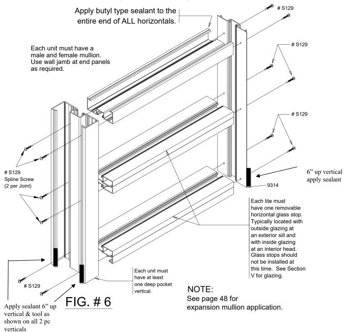
The shear block system is a fabrication and erection method that permits the preassembly of single units in the shop or at the job site. These units are joined with shear blocks and installed as an assembled unit in the opening on top of any sill flashing that is used. Shear block joinery will be used at any immediate door frame.
