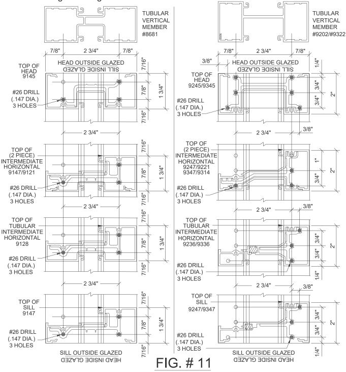
USE BLOCKED OUT HOLE LOCATIONS FOR SHEAR BLOCK APPLICATIONS
