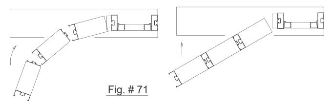
EFCO requires the use of at least a 3" long piece of adaptor at all fastener locations, FS92 or FV58 at S401, FS93 or FV59 at S402, and FU99 or FV59 at S403.
