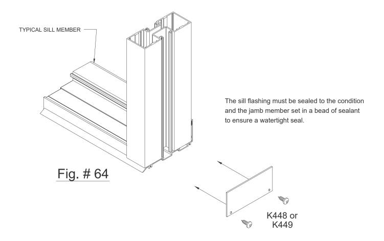
Incorporating the sill flashing end caps will complement the sealing procedure.
