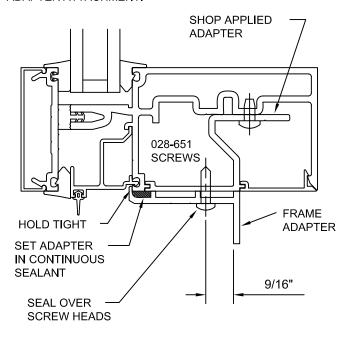
APPLY ADAPTERS TO ALL 4 SIDES AND SEAL CORNERS AS SHOWN.
