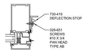
WITH THE VENT OPEN, LOOSEN SCREWS SO STOP WILL SLIDE. THEN SLIDE DEFLECTION STOP TOWARDS THE INTERIOR. CLOSE VENT AND LOCK. OPEN THE VENT CAREFULLY AND TIGHTEN DEFLECTION STOP SCREW.
