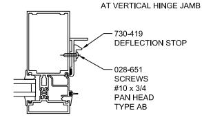
APPLY DEFLECTION STOP. USING HOLES IN ADAPTERS DRILL HORIZONTAL WITH #26 DRILL 0.147 DIA. AND APPLY WITH 028-651 SCREWS. ADJUST STOP ALL THE WAY TO THE EXTERIOR AND SNUG TIGHTEN SCREWS. ADJUSTMENT WILL BE REQUIRED AFTER THE VENT IS INSTALLED.
