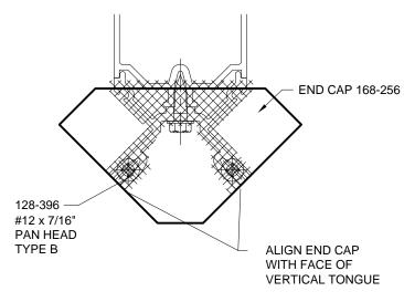
APPLY SEALANT INTO SCREW RACE TO SEAL END OF FASTENER AT TOP AND BOTTOM. TOOL SEALANT AROUND ALL EDGES. SEAL OVER FASTENER HEAD.
